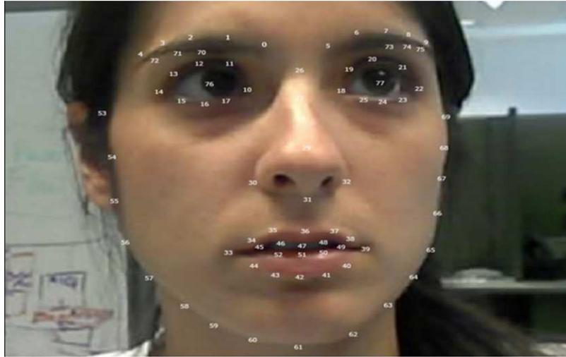
Figure 4. Intel® Real Sense™ SDK Landmark Data
