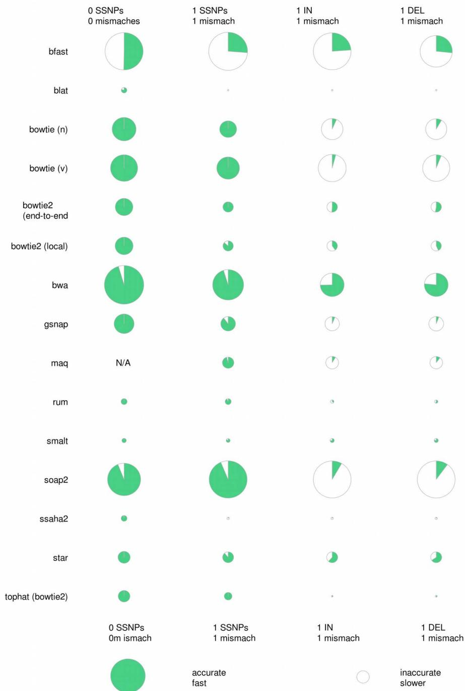
Figure 5. The accuracy and throughput of each short read alignment tool evaluated for genome exon alignment using different IM/INDEL and mismatch metrics. The size of the pie chart is proportional to the throughput achieved by the alignment tool, while the green slicing of the pie chart represents the alignment accuracy.
