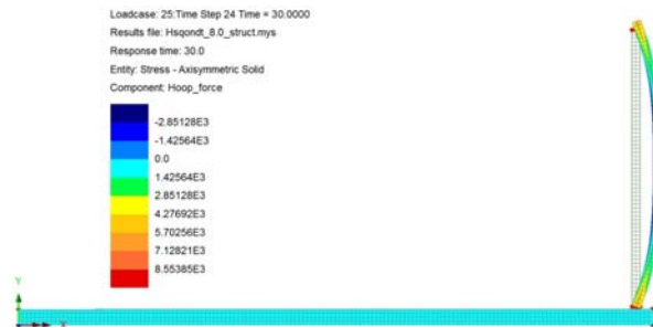
Figure 4: Finite element model showing a deformed contour of hoop forces
