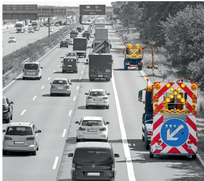
Figure 1. A protective vehicle safeguarding a road maintenance vehicle in front of itself (Hessen Mobil)
