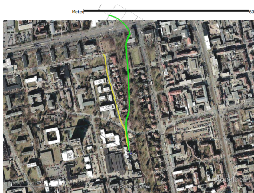
Figure 4: Results of GPS (yellow track, left) and INS (green track, right) Measurements in Comparison (CCASS, 2012)
