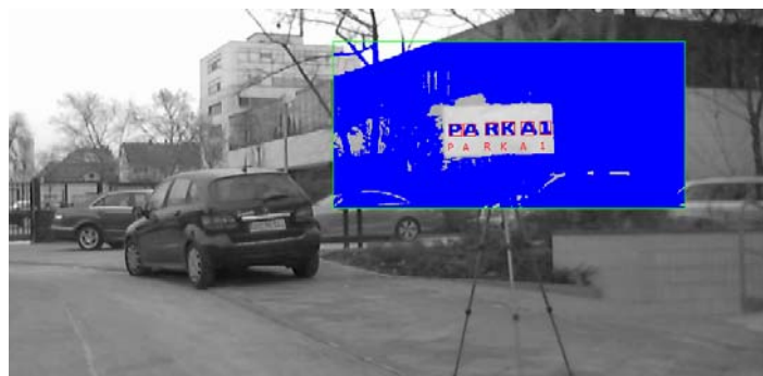
Figure 5: Sample Result of Road Sign Recognition from In-Car-Video with a CCASS-Software (CCASS, 2012)
