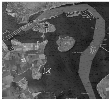
Figure 3: A vessels anomaly is located outside the standard shipping lane (far left circular cluster). The simulated vessel indicated no AIS data. Entered the ports restricted area and returned back to open water without port authority.
